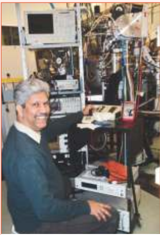
(VHF) PECVD/HWCVD UHV 5 chamber cluster tool
