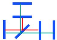
**State 4** : The remaining ETM is controlled and the carrier resonates in both arms and the recycling cavity.
