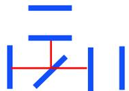
**State 2** : The power recycling cavity is held on a carrier anti-resonance. In this state the sidebands resonate in the recycling cavity.
