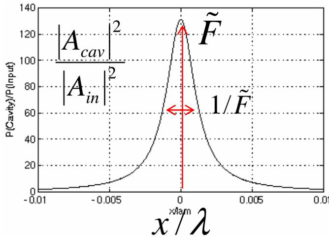
$$A_{cav} = A_{in} \frac{t_{ITM}}{1 - r_{ITM} r_{ETM} e^{i\phi}}$$
