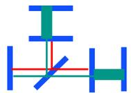
**State 5** : The power in the IFO has stabilized at its operating level. This is the ending point for lock acquisition.
