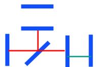
**State 3** : One of the ETMs is controlled and the carrier resonates in the controlled arm.
