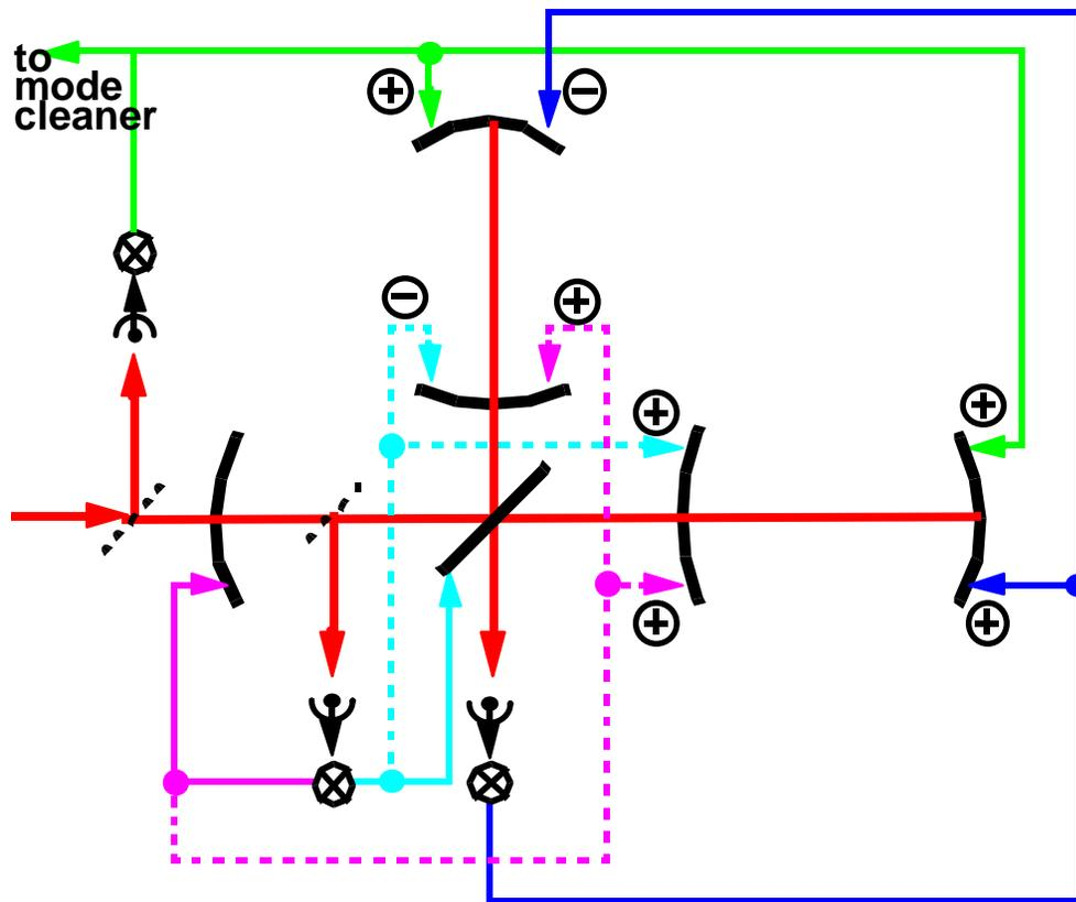
example: cavity length sensing & control topology
