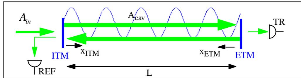
$$A_{cav} = A_{in} \frac{t_{ITM}}{1 - r_{ITM} r_{ETM} e^{i\phi}} \quad \tilde{F} = \left( \frac{t_{ITM}}{1 - r_{ITM} r_{ETM}} \right)^2 \approx \frac{4}{t_{ITM}^2}$$
