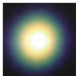
White light continuum from Water/D 2 O under ps pumping
