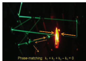
Phase-conjugate geometry of degenerate four wave mixing
