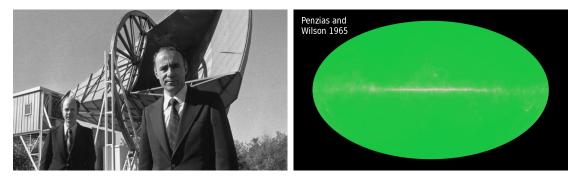
The horn antenna used by Penzias and Wilson (on the left) and the CMB as observed by them (on the right).
