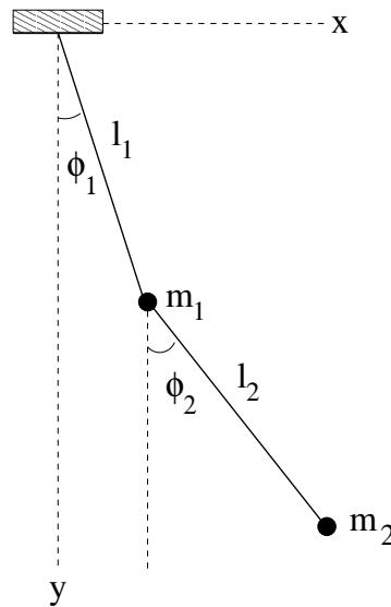
(b) a simple pendulum of mass  $m_2$ , with a mass  $m_1$  at the point of support which can move on a horizontal line lying in the plane in which  $m_2$  moves as shown in the figure below,
